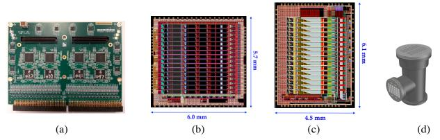
Fig. 6 (a) FEMB used for cold evaluation tests of FE ASIC. (b) 16-channel low power and low noise cold analog front end ASIC. (c) 16-channel low power and 12-bit 2Msps ADC ASIC. (d) Schematic picture of feedthrough. Figures (a), (b), (c) are from [11], and (d) is from [12].
