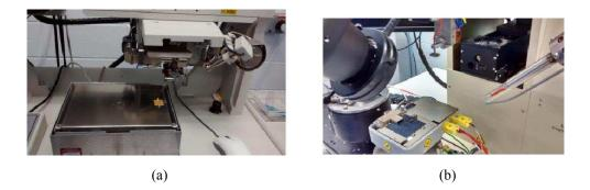
Fig.4 (a) West Bond Bump Bonder: The device that deposits the bumps. (b)SEC Model 860 Eagle Omni Bonder: Aligns the two surfaces and applies heat and compression
