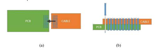
Fig.5 (a) Connecting PCB and Kapton cable by pressing fit a pin between the two. (b) Wire bond between PCB and the cable. Figures are extracted from [9].
