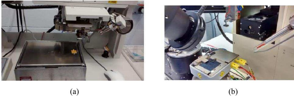
Fig.4 (a) West Bond Bump Bonder: The device that deposits the bumps. (b) SEC Model 860 Eagle Omni Bonder: Aligns the two surfaces and applies heat and compression
