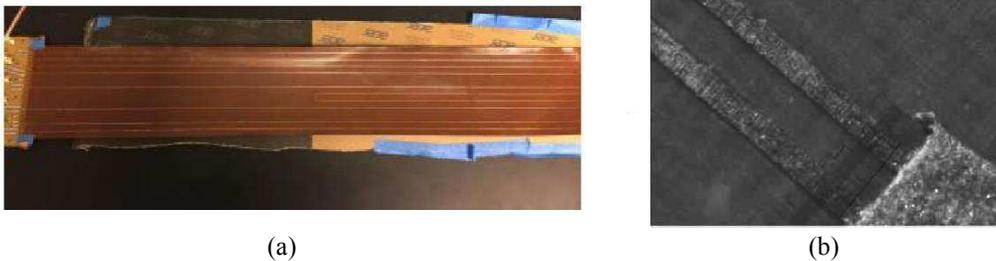
Fig. 1 (a) 3 pairs of transmission lines under test in the preliminary study. (b) Coupled transmission lines under microscope. No apparent discontinuities or tapering have been observed.
