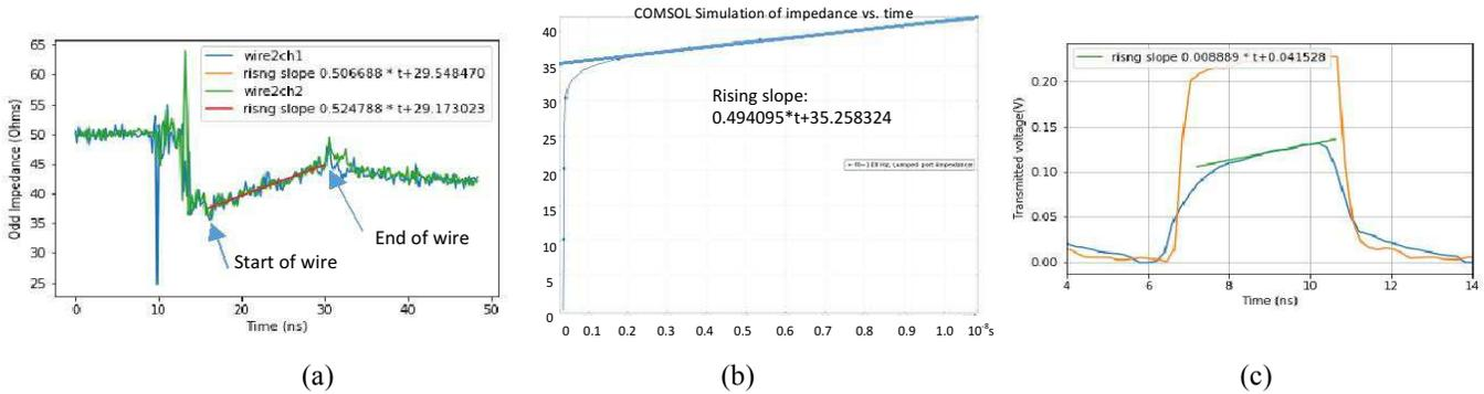
Fig. 2 (a) TDR measurements of the cable's impedance. The characteristic impedance is measured to be  $37\Omega$ . The slope in the impedance vs. time is caused by resistive loss in the cable. (b) COMSOL simulation of measurement (a). A similar slope shows up in the TDR simulation. (c) Measured input (orange) and transmission pulse signal (blue). The gap between the two is due to loss and impedance mismatch between the microstrip transmission lines and the signal generator's coaxial cables.
