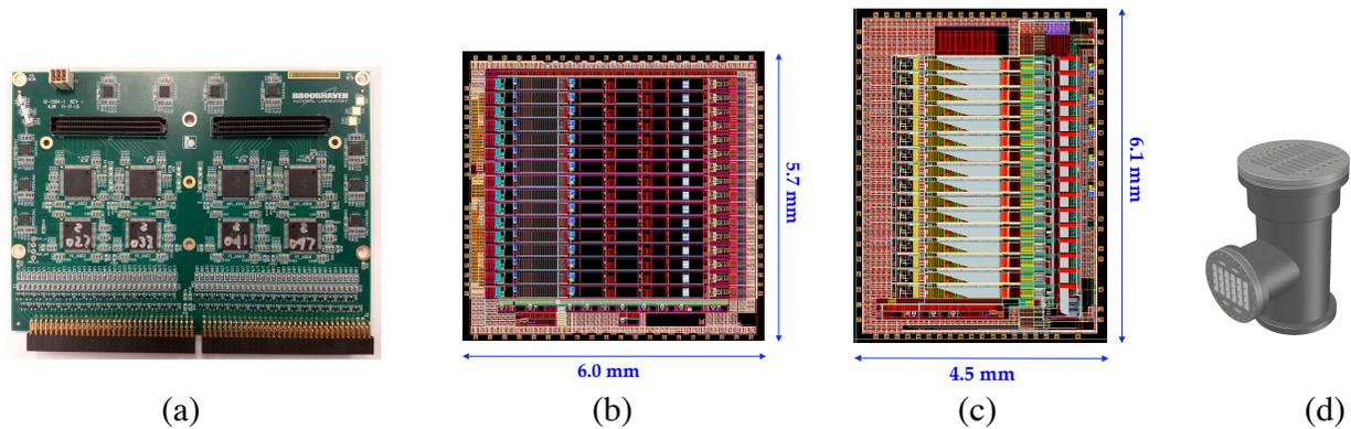
Fig. 6 (a) FEMB used for cold evaluation tests of FE ASIC. (b) 16-channel low power and low noise cold analog front end ASIC. (c) 16-channel low power and 12-bit 2Mps ADC ASIC. (d) Schematic picture of feedthrough. Figures (a), (b), (c) are from [11], and (d) is from [12].
