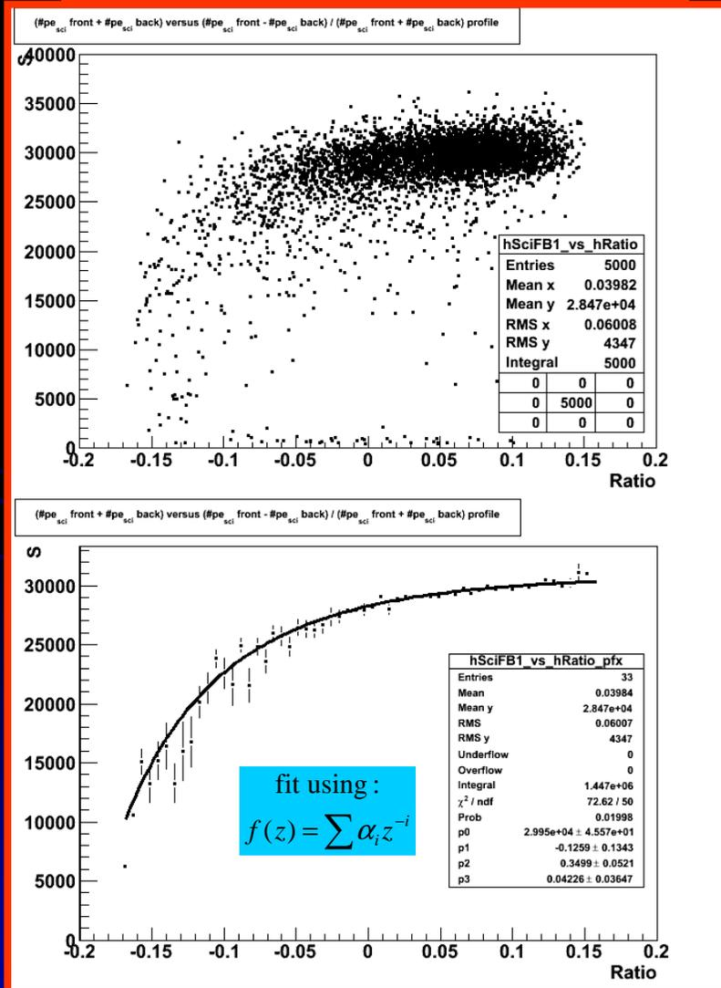
Corrected scintillating signal
