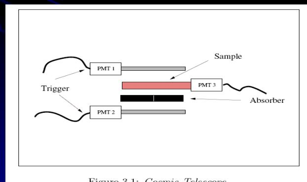
Figure 3.1: Cosmic Telescope.
