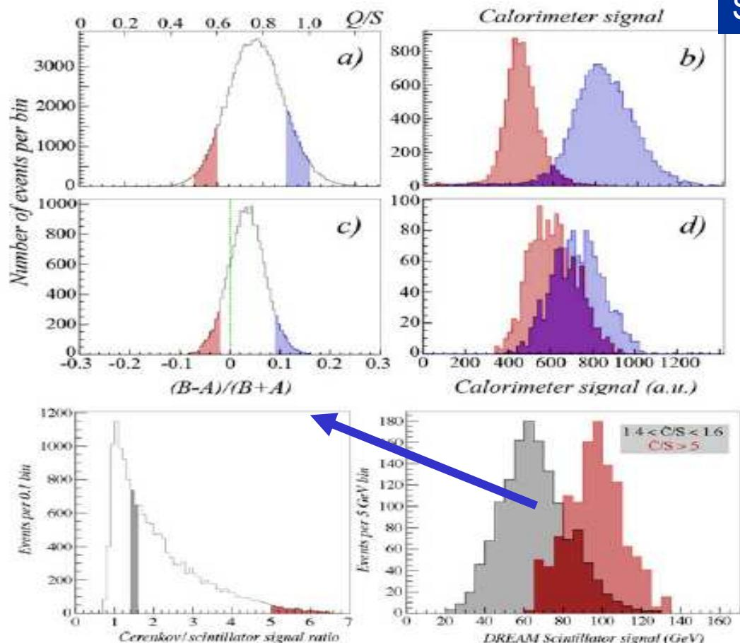
Separation Efficiency between S & C components
