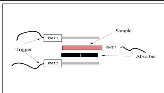
Figure 3.1: Cosmic Telescope.
