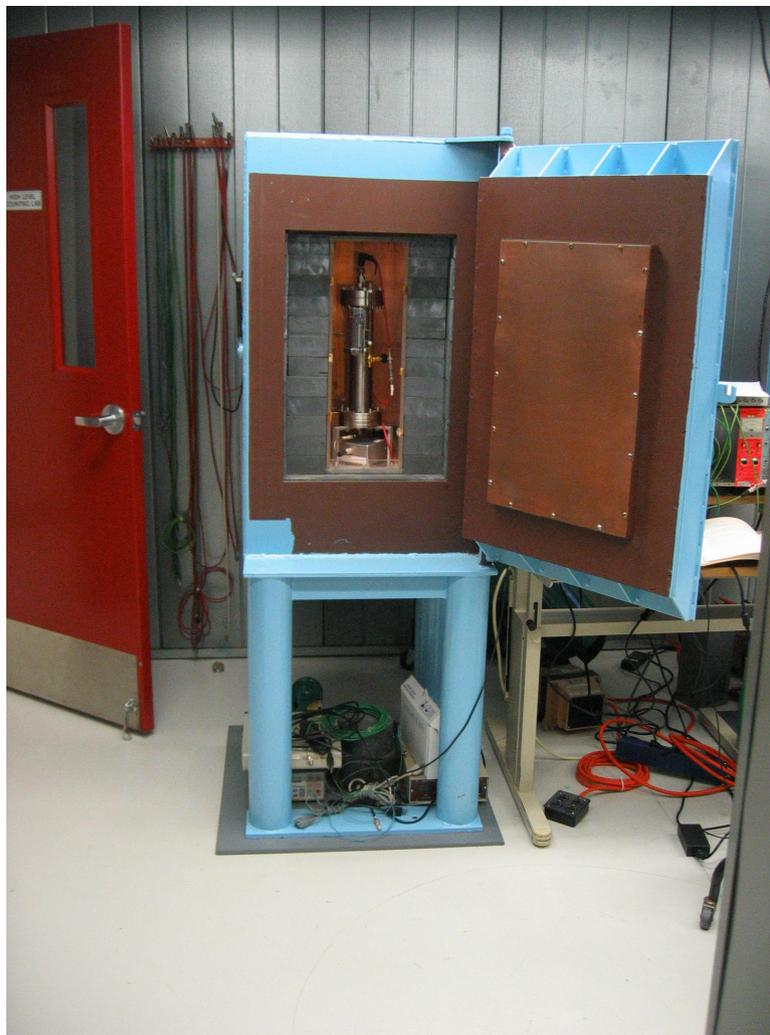
59.5 keV X-rays in Ionization Chamber
