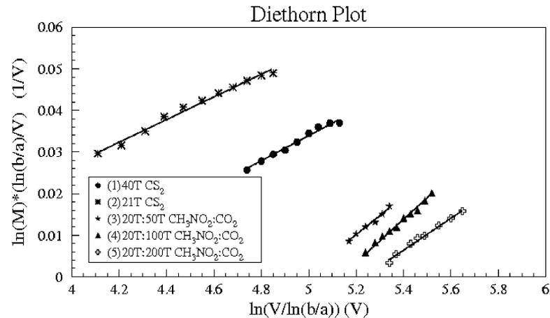
Figure 4.20: Diethorn plots for several negative ion gas mixtures studied in the present work.
