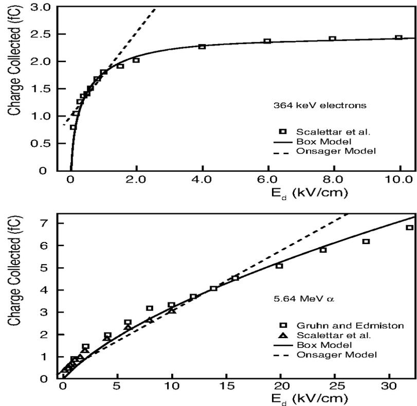
Dense ionization is hard to collect before recombination occurs.
