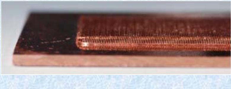
Footprint h.t.c.'s up to 270'000 W/m<sup>2</sup>K for high aspect microchannels and h.t.c.'s increase with heat flux
