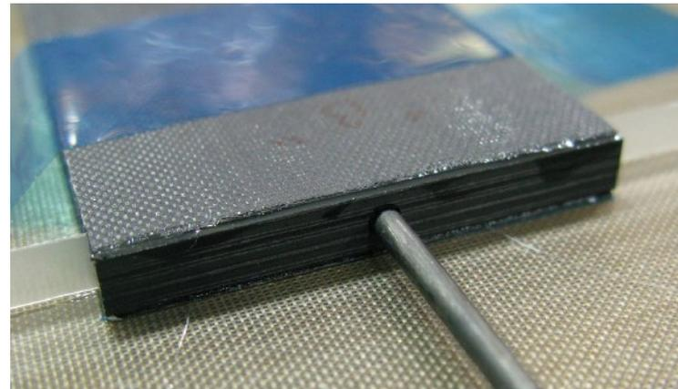
Pixel stave core with Ti pipe
