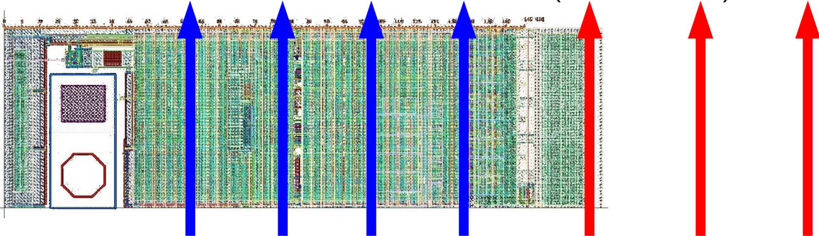
Power distribution and shield on top metals. Only vertical - no analog/digital crossing
