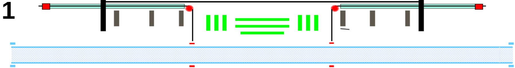
Insert support rod and disconnect cable system; cut off one flange
