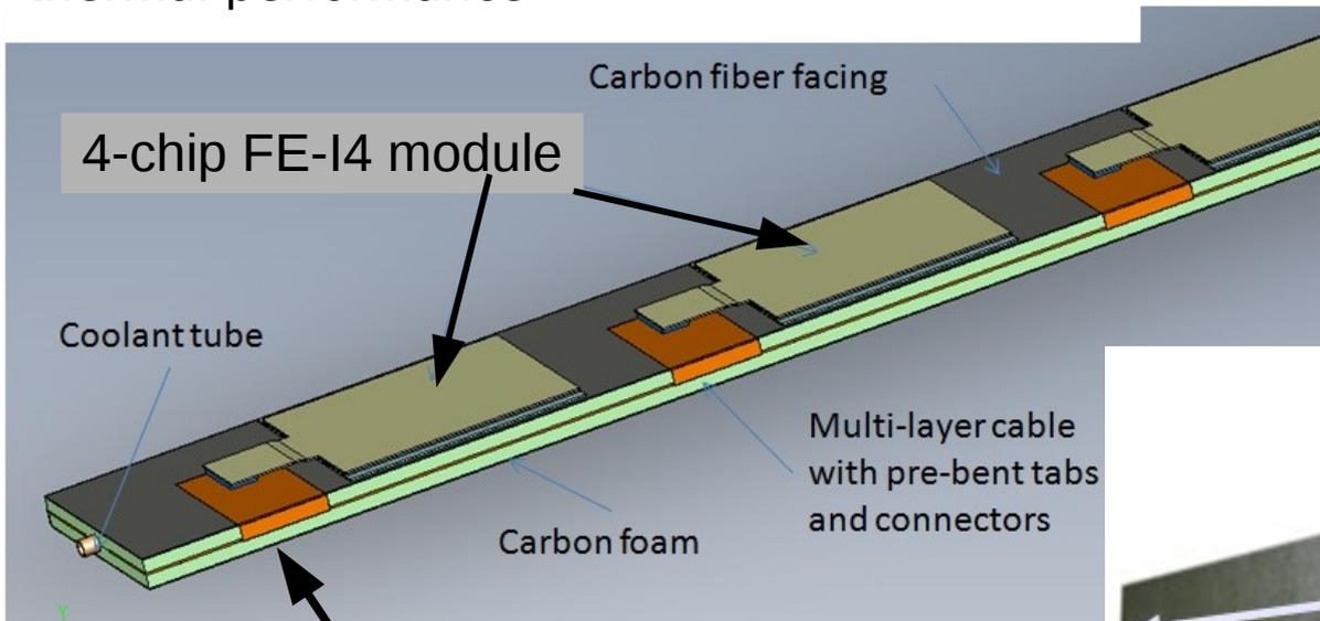
First thermal prototype Bus cable (similar concept to silicon strip staves) glued on top of mechanical stave
