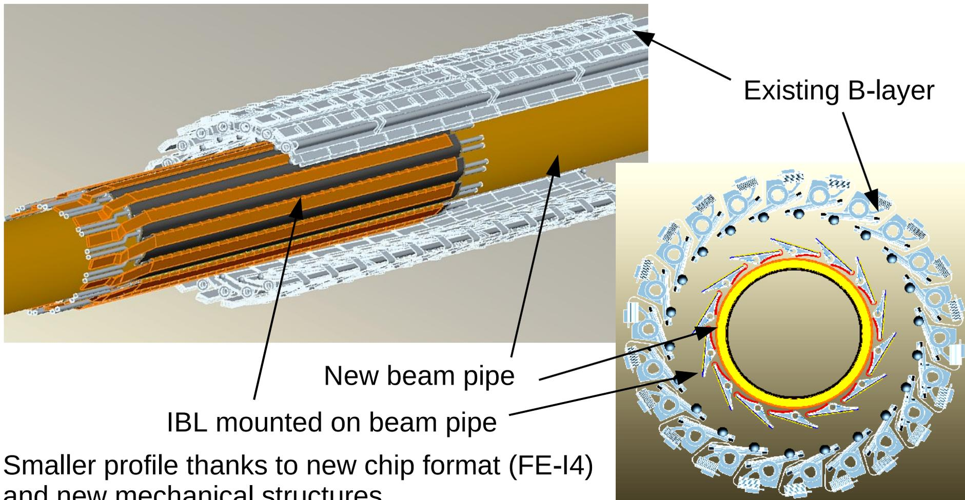
Smaller profile thanks to new chip format (FE-I4) and new mechanical structures.
