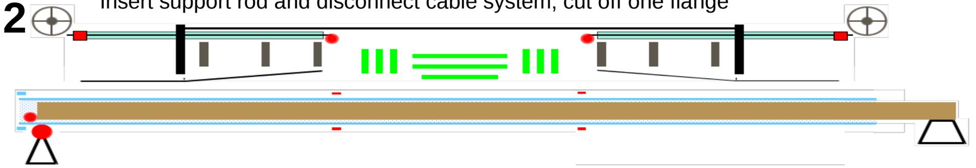
Slide out old beam pipe and slide in new one with IBL and IBL services on it; remove rod
