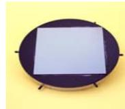
3 inch diameter platen allows growth on one 6x6 cm substrate
