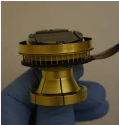
Visible FPA sensor subassembly
