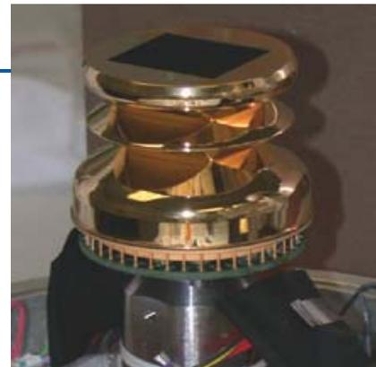
Infrared FPA sensor subassembly
