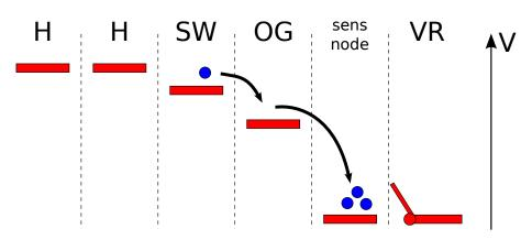
Move the change to the SN and measure the shift in the voltage  $\,$
