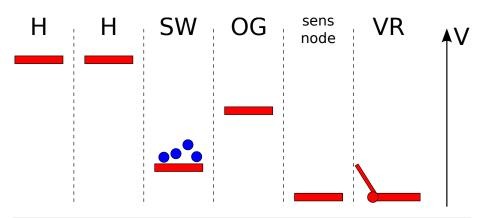
Disconnect the SN so it's floating. Measure the baseline voltage in the SN.
