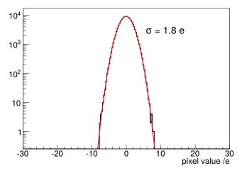
2 e<sup>-</sup> readout noise roughly corresponds to 50 eV energy threshold
