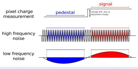
excellent for removing high frequency noise but sensitive to low frequencies
