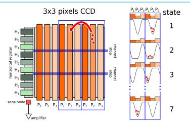
capacitance of the system is set by the SN: C=0.05pF ightarrow  $3\mu$ V/e
