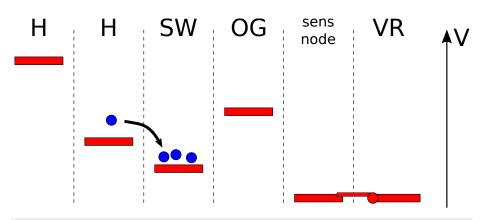
Accumulate the charge in the SW and reset the SN voltage
